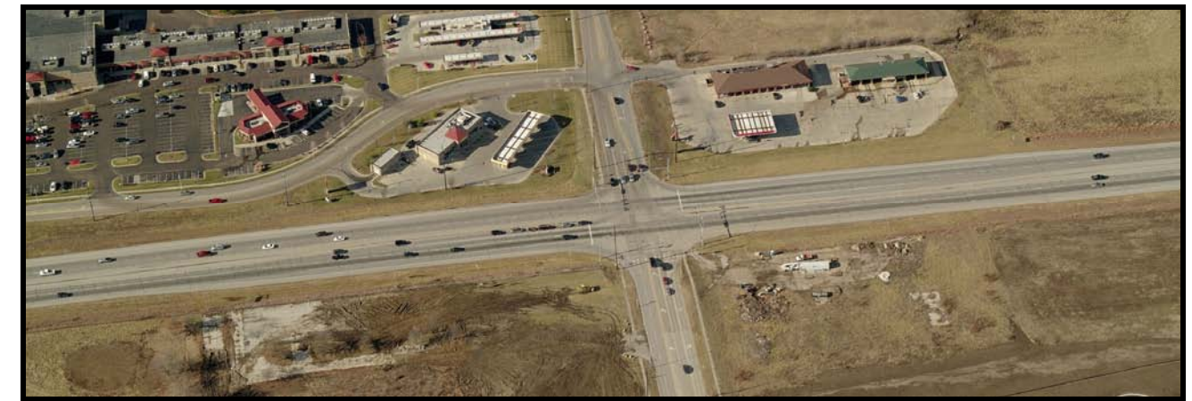
Typical Urban Expressway Intersection with Access Roads
