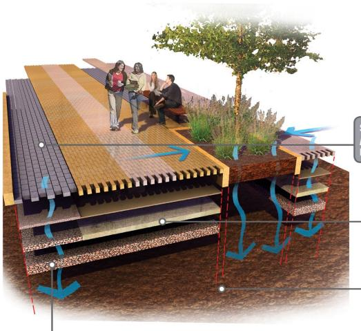
Spaces between the **permeable pavers** direct water to a series of layers below the pavement sub base.
