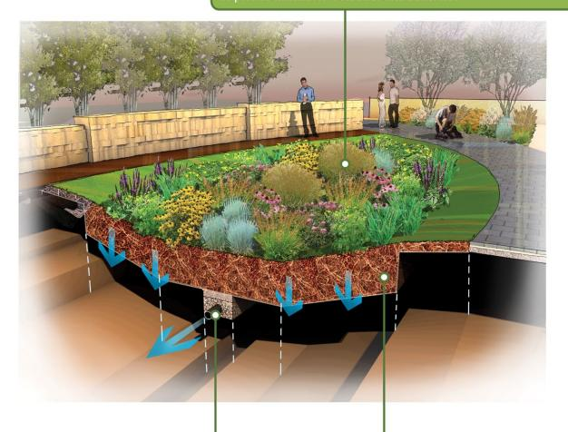
To help remove excess water from the stormwater planter, the *under drain* insures that water will not pond on the surface for extended periods of time.
