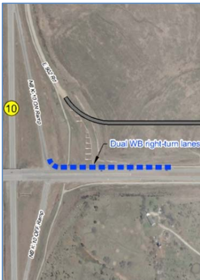
right-turn lanes for westbound US-40 at east ramp terminal
