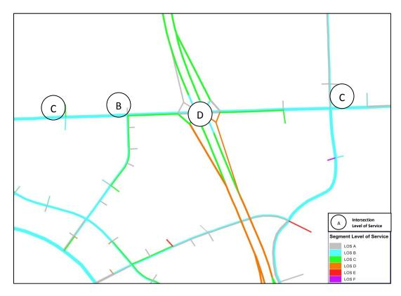
Figure 5.3.3 – Roadway and Intersection Levels of Service for Single Point Urban Interchange Configuration at Parallel Parkway with State Avenue Corridor Improvements Design Year 2040 Weekday PM Peak Hour Traffic Volumes
