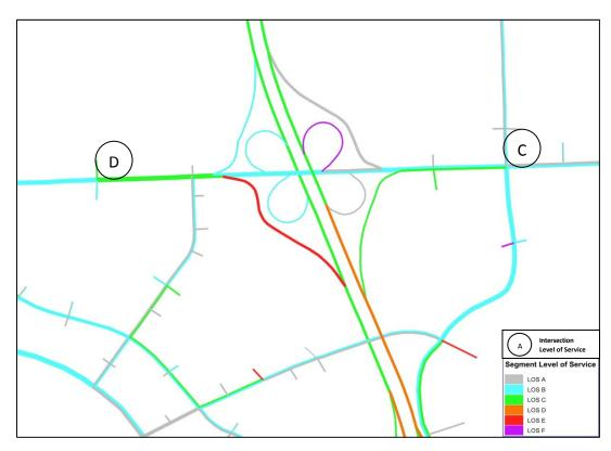
Figure 5.2.1 – Roadway and Intersection Levels of Service for No Build Design Year 2040 Weekday PM Peak Hour Traffic Volumes
