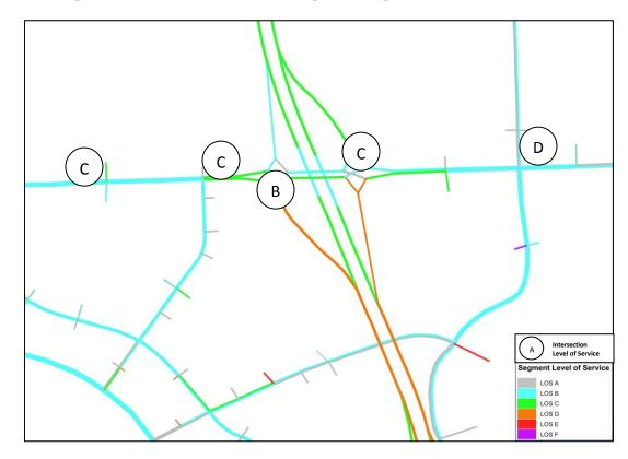
Figure 5.3.4 – Roadway and Intersection Levels of Service for Diverging Diamond Interchange Configuration at Parallel Parkway with State Avenue Corridor Improvements Design Year 2040 Weekday PM Peak Hour Traffic Volumes
