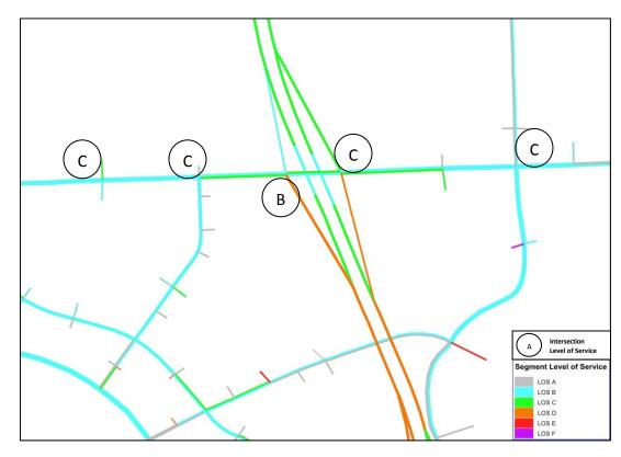
Figure 5.3.2 – Roadway and Intersection Levels of Service for Standard Diamond Interchange Configuration at Parallel Parkway with State Avenue Corridor Improvements Design Year 2040 Weekday PM Peak Hour Traffic Volumes
