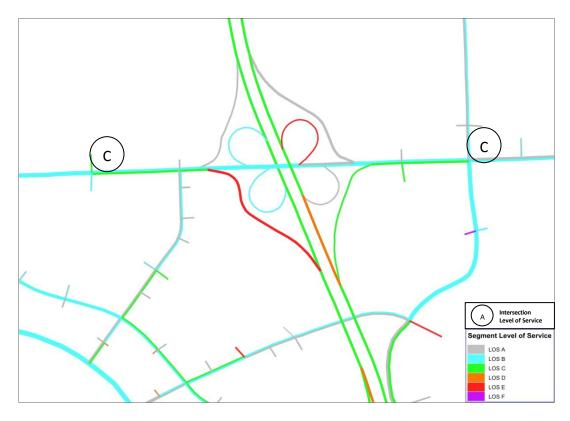
Figure 5.3.1 – Roadway and Intersection Levels of Service for No Build on Parallel Parkway with State Avenue Corridor Improvements Design Year 2040 Weekday PM Peak Hour Traffic Volumes
