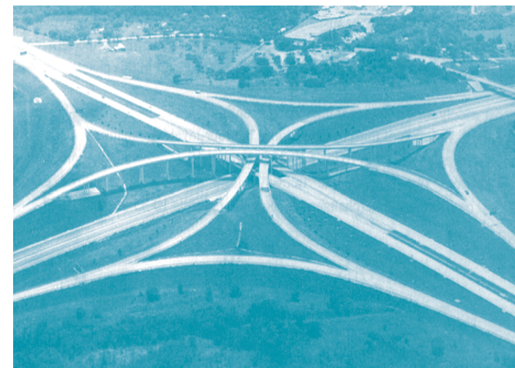
Example of a four level interchange
