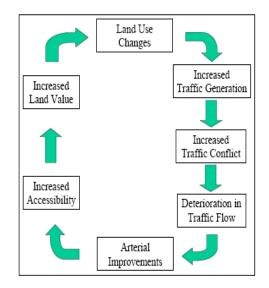
roads that are designed to go to and by commercial sites are often designed to provide sufficient flow and access to the development. In fact, KDOT's Access Spacing Criteria consider land use and level of development among the factors in determining appropriate access spacing.
