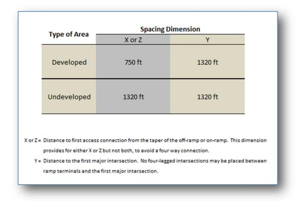
Figure 10: Minimum spacing for freeway interchange with two-lane crossroads (KDOT Access Management Policy)
