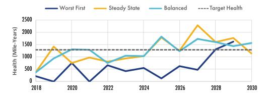
As shown, while all three scenarios surpass the target pavement health in the long-term, the Desired SGR (Balanced) scenario has the smallest gap over the entire projection period.
