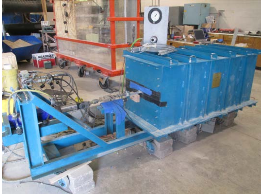
Figure 3.2: RJH Pullout Test Apparatus
