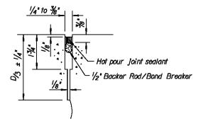
Make the initial saw cut at 1/8 inch (D/3  $\pm 1/4$  inch). Make the 3/8 inch saw cut in a separate operation after the concrete has gained sufficient strength to avoid spalling.
