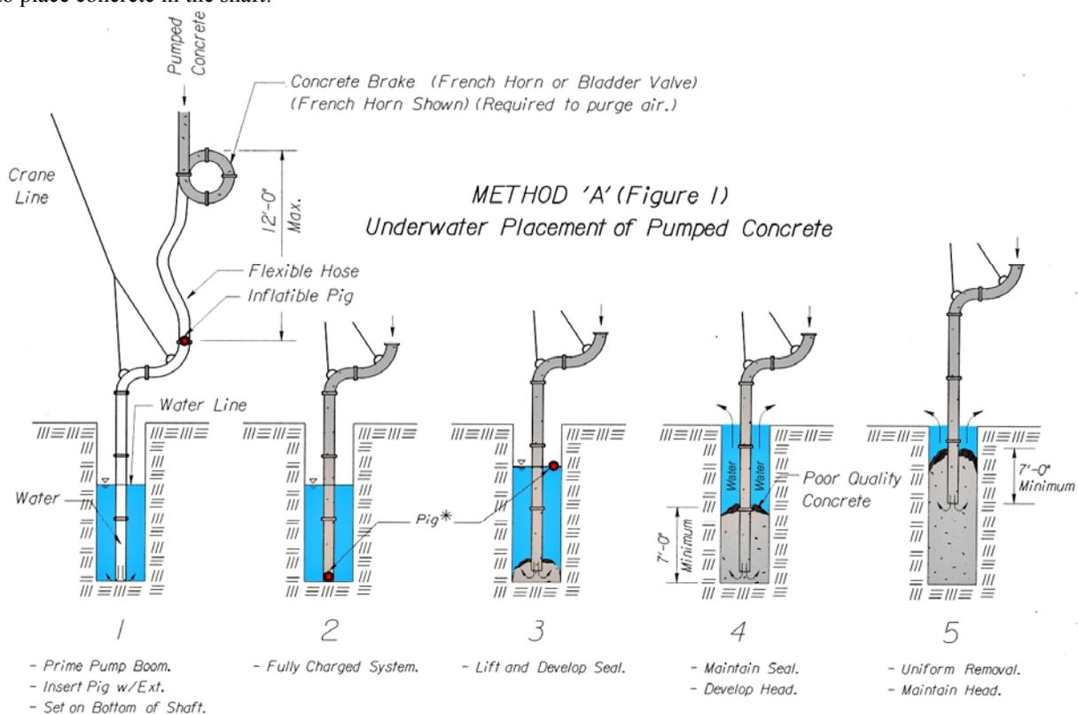
**Method A (Figure 1):** Use a pump and extension tube, with a pig separating the ground water and concrete, to place concrete into the shaft. Install a concrete brake (e.g. bladder valve or French horn) at the end of the pump boom to purge the air from the pump line. Fully charge the boom with concrete (no air gaps) then install the pig in the top of the extension tube.
