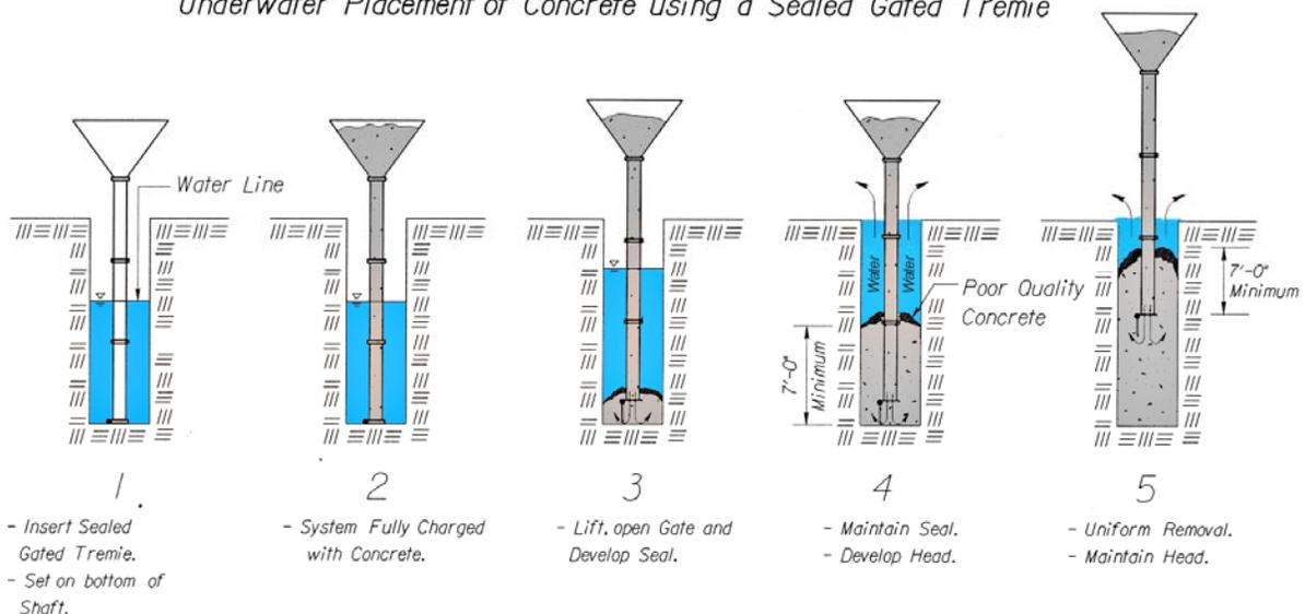
**Method C (Figure 3):** Use a tremie tube, with a sealed gate separating ground water and concrete, to place concrete in the shaft. Fully charge the tremie tube and hopper, then raise the tremie tube by 1 tremie diameter and seal the discharge end of the tremie tube with the fresh concrete.
