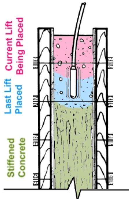
**Figure 21: Placement and Initial Set of Concrete**
