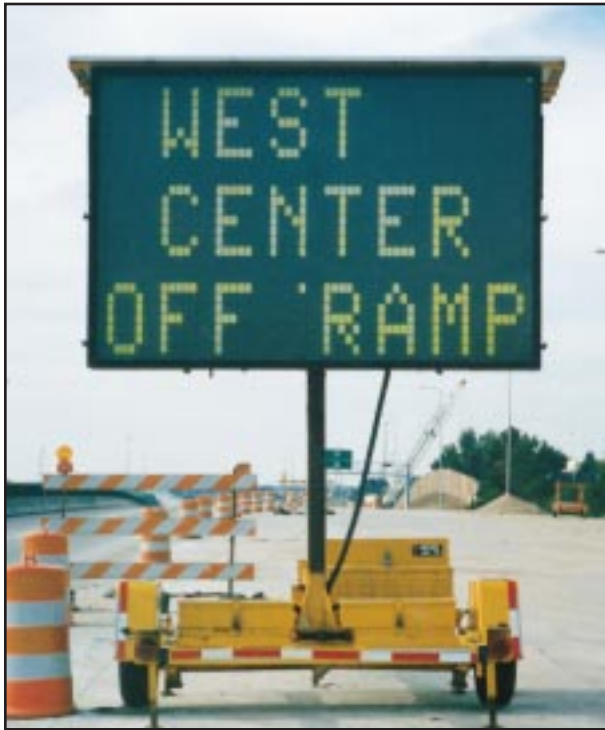
West Center off-ramp variable message sign
