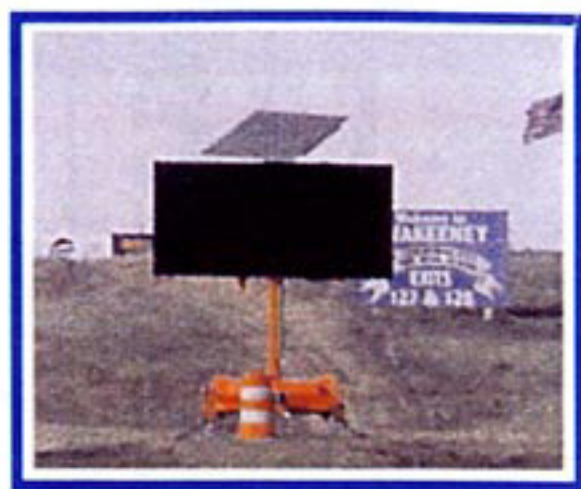
VMS (Variable Message Sign) in District 3 along I-70.
