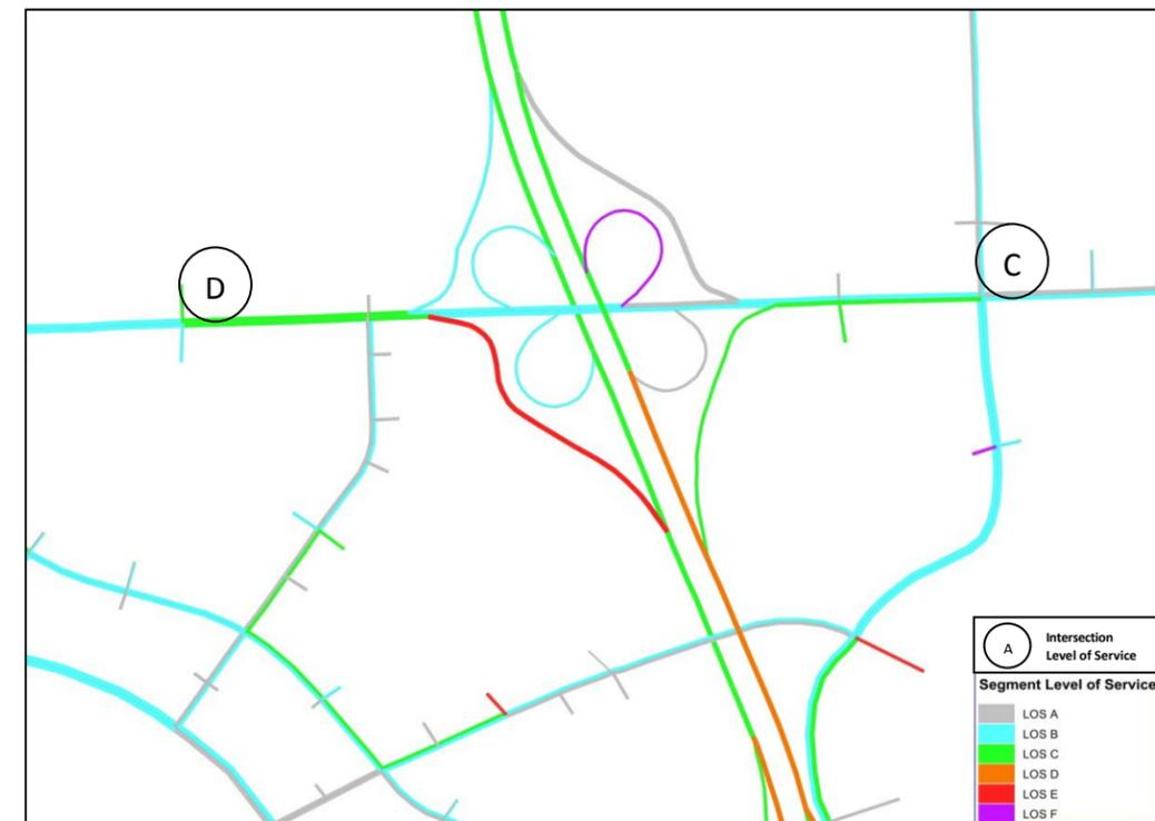
**Figure 5.2.1 – Roadway and Intersection Levels of Service for No Build Design Year 2040 Weekday PM Peak Hour Traffic Volumes**
