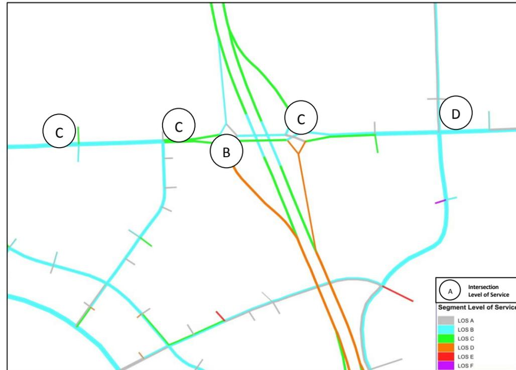
**Figure 5.3.4 – Roadway and Intersection Levels of Service for Diverging Diamond Interchange Configuration at Parallel Parkway with State Avenue Corridor Improvements Design Year 2040 Weekday PM Peak Hour Traffic Volumes**
