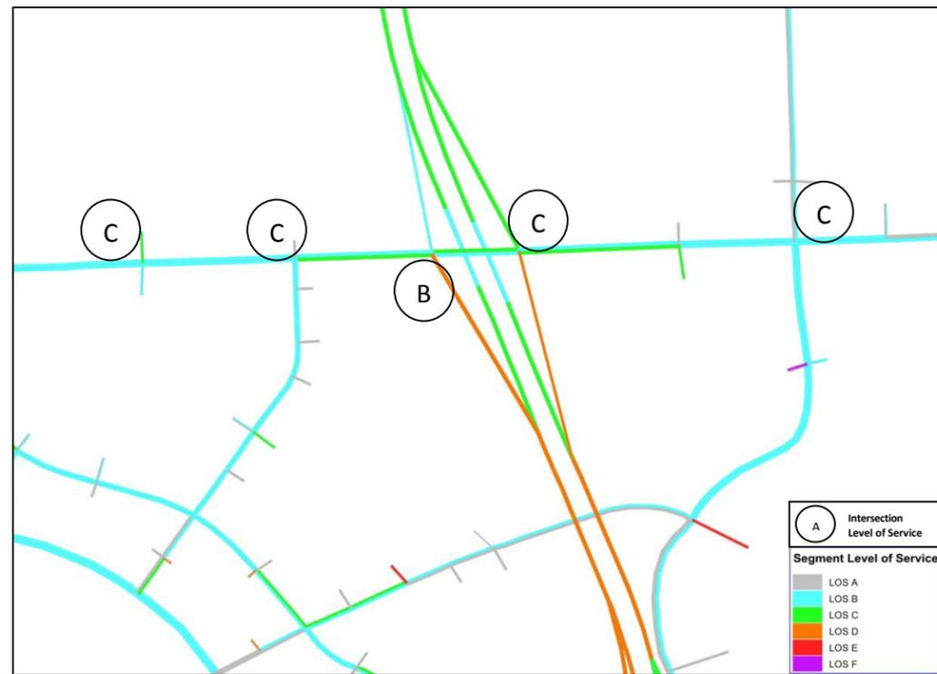
**Figure 5.3.2 – Roadway and Intersection Levels of Service for Standard Diamond Interchange Configuration at Parallel Parkway with State Avenue Corridor Improvements Design Year 2040 Weekday PM Peak Hour Traffic Volumes**
