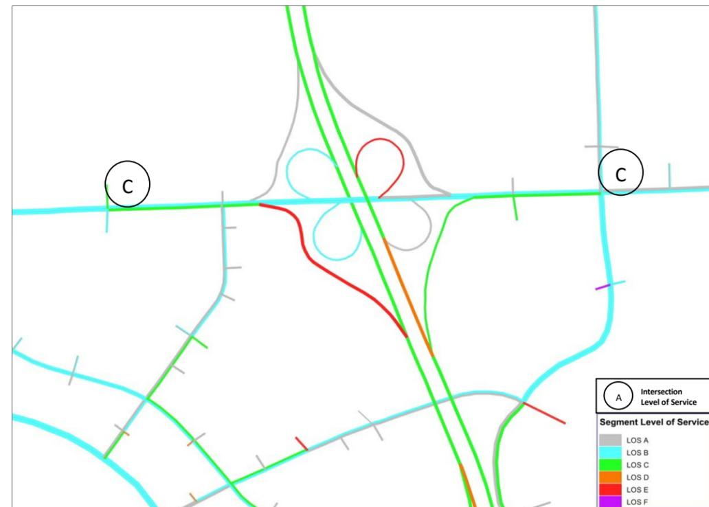
**Figure 5.3.1 – Roadway and Intersection Levels of Service for No Build on Parallel Parkway with State Avenue Corridor Improvements Design Year 2040 Weekday PM Peak Hour Traffic Volumes**
