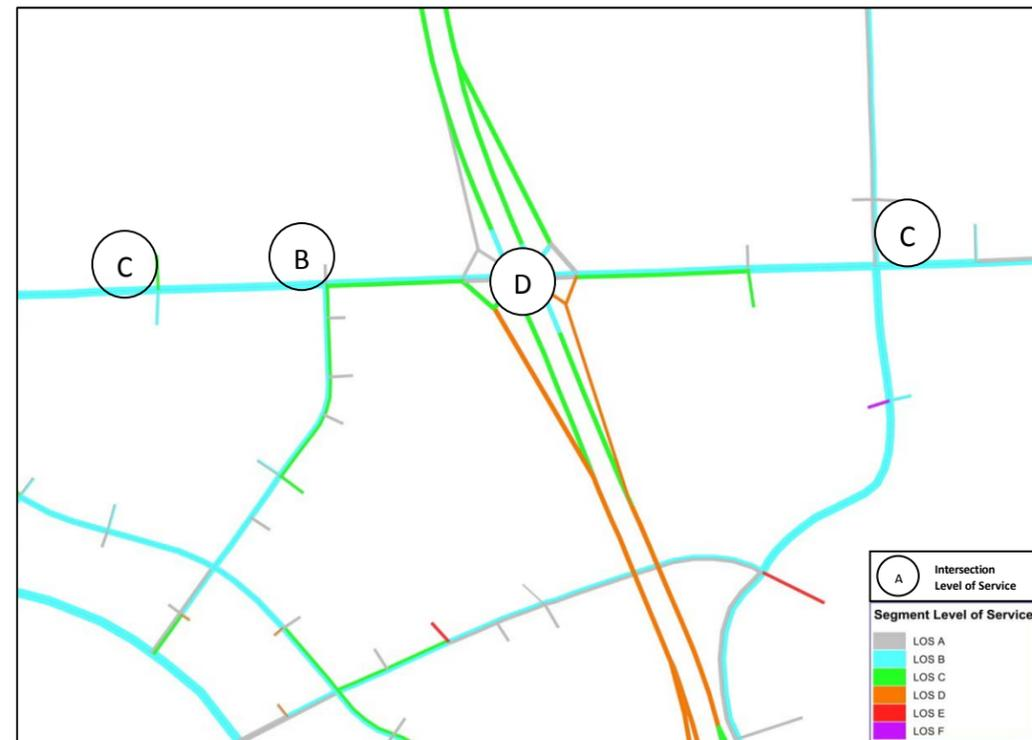
**Figure 5.3.3 – Roadway and Intersection Levels of Service for Single Point Urban Interchange Configuration at Parallel Parkway with State Avenue Corridor Improvements Design Year 2040 Weekday PM Peak Hour Traffic Volumes**
