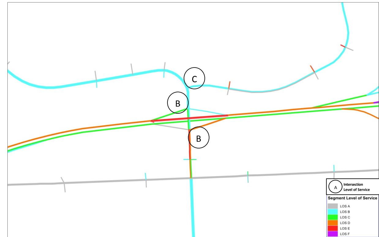
Figure 7.3.2 – Roadway and Intersection Levels of Service for 110 th Street with State Avenue Corridor Improvements and I-70 / I-435 Interchange Improvements
