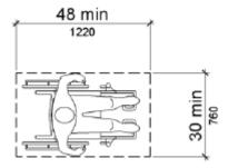
305.4 Knee and Toe Clearance. Unless otherwise specified, clear floor or ground space shall be permitted to include knee and toe clearance complying with 306.
