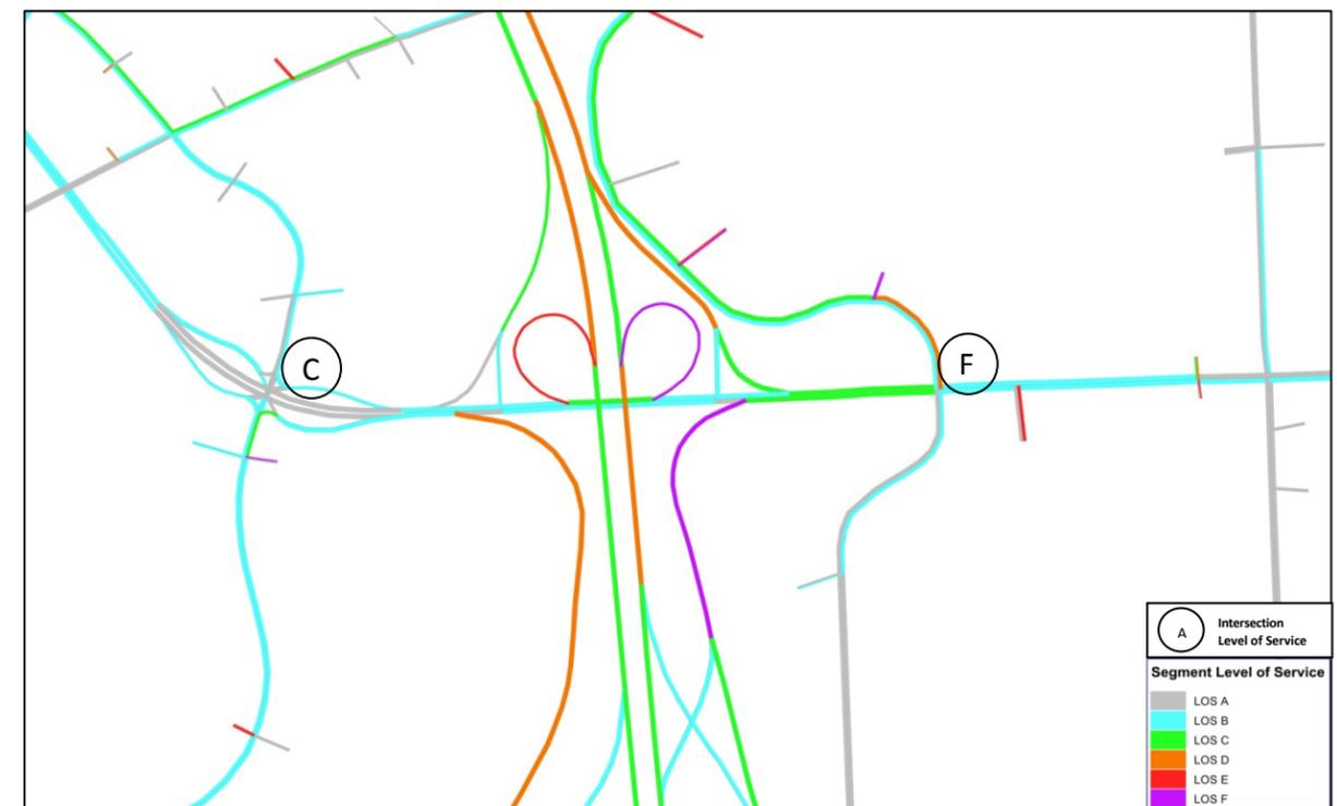
**Figure 4.4.2 - Roadways and Intersection Levels of Service for Single Point Urban Interchange at Village West Parkway Design Year 2040 PM Peak Hour Traffic Volumes**
