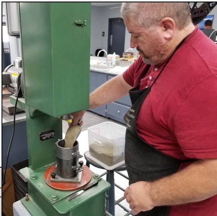
**Above:** Ken Slack, Engineering Technician with KDOT's District Five lab, scoops soil for compaction testing.
