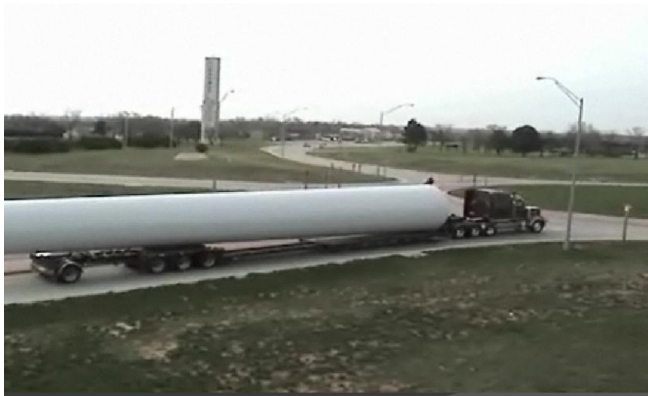
FIGURE 5.4 Wind Generator Tower Section Going through Kansas Roundabout at Florence
