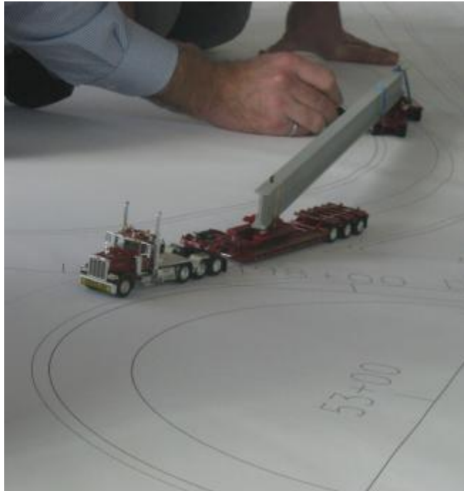
FIGURE 5.35 Using the Model of an OSOW to Layout Needed Accommodating Space in a Roundabout
