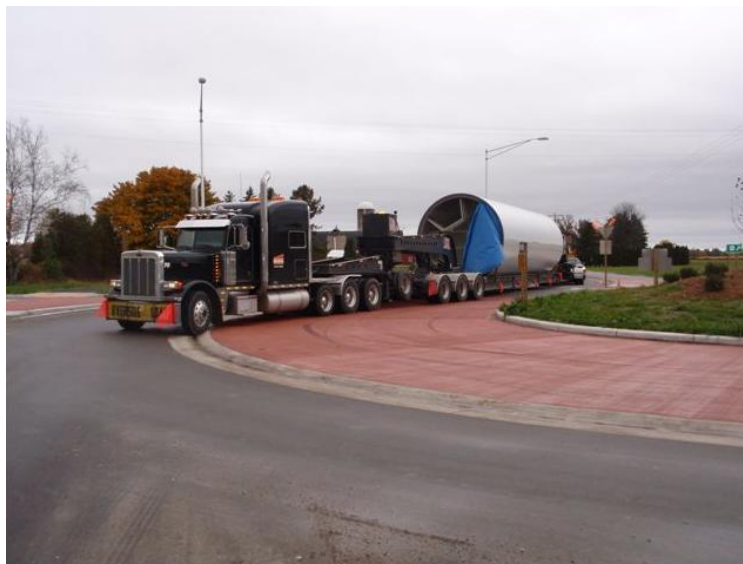
FIGURE 5.11 Advantage of Wide Truck Apron in Arizona
