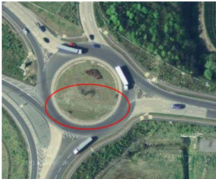
FIGURE 5.9 An Example from the UK of a Turf-Stabilized Center Island
