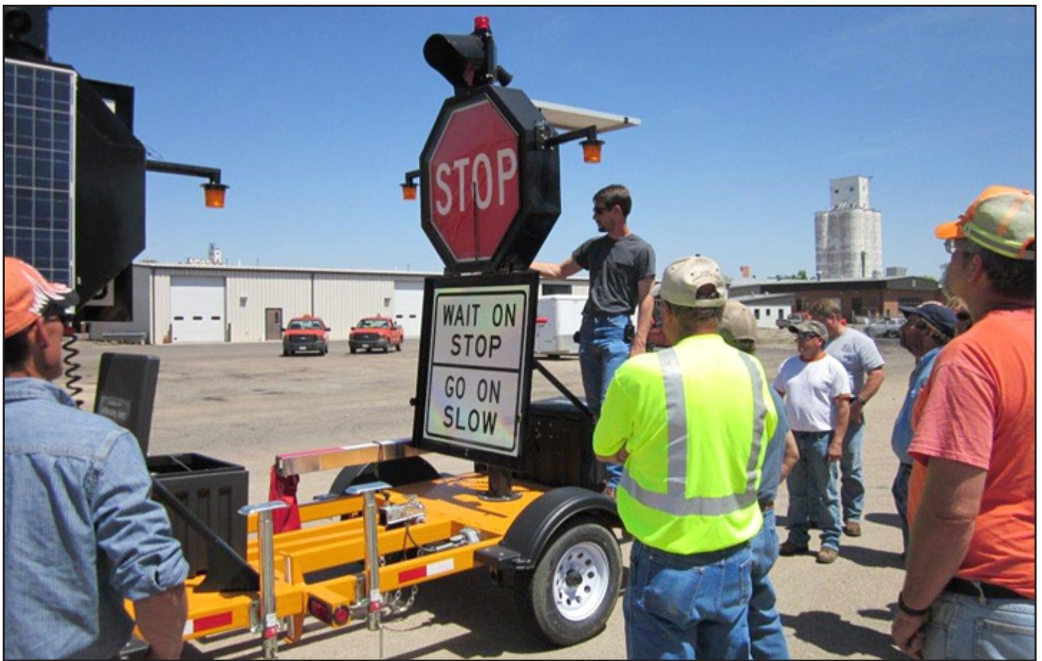
KDOT employees in District Three participate in a training session on using the Automatic Flagger Assistance Device in work zones.
