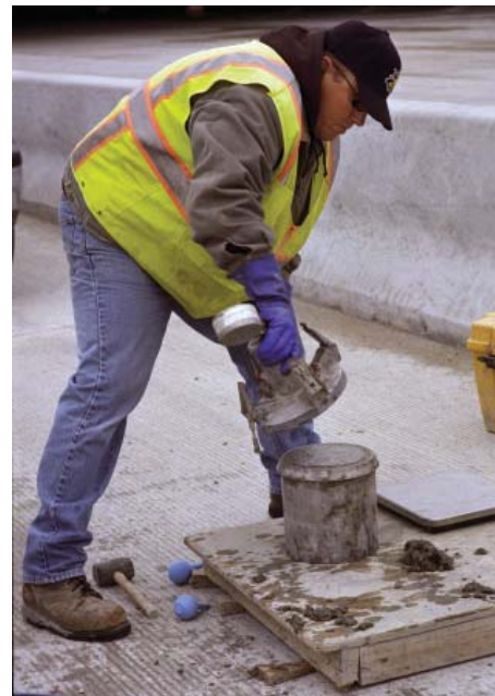
An inspector performs an air content test on a concrete sample on U.S. 54/400 in Wichita.
