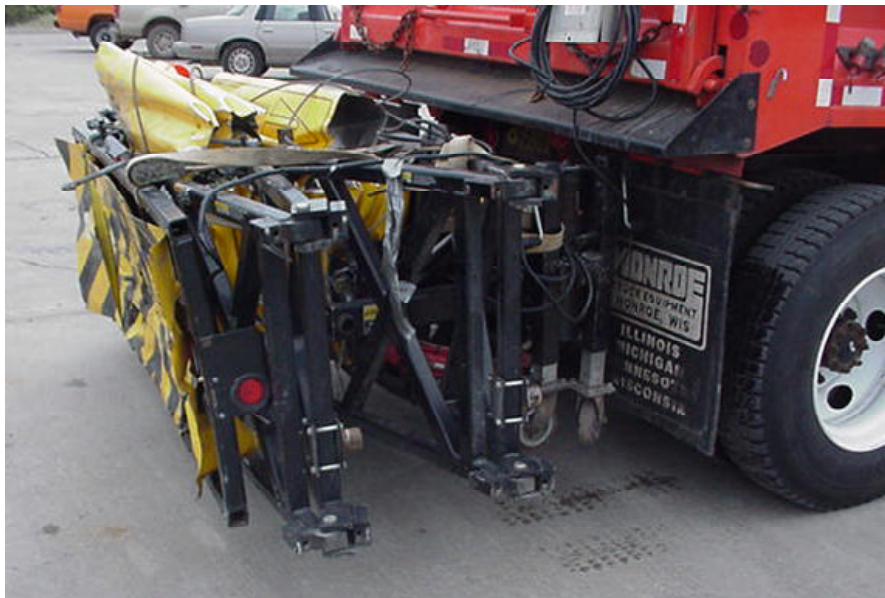
This attenuator did its job when it was hit by a motorist on I-35 last month. Although it was damaged beyond repair, the important thing is the motorist survived and no KDOT personnel were hurt.
