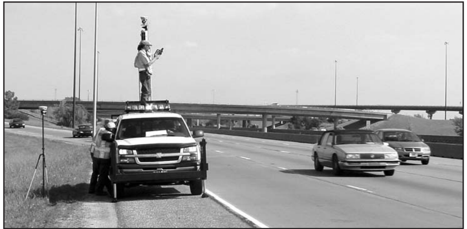
Survey information can be gathered on the side of the highway when using a Cyrax laser scanning system.
