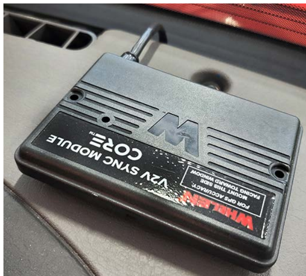
Warning lights on the truck (above) can be synchronized by operators with this box (below) to other warning lights in the area. Photos by Tracy Statton, District Five
