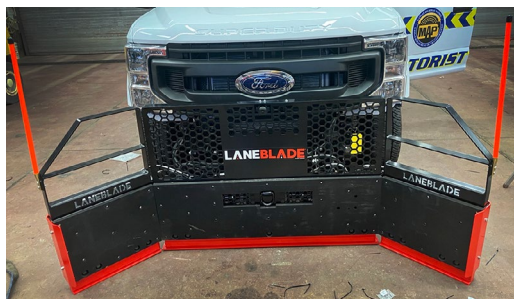
Above left, the LaneBlade system installed on a Wichita-area Motorist Assist vehicle. Right, the DebrisClear system that will be used by the KHP in the Kansas City area. Photos by Brent Engelland, Hutchinson, and Kate Craft
