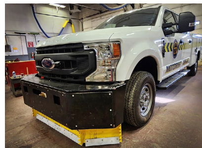
Above left, the LaneBlade system installed on a Wichita-area Motorist Assist vehicle. Right, the DebrisClear system that will be used by the KHP in the Kansas City area. Photos by Brent Engelland, Hutchinson, and Kate Craft
