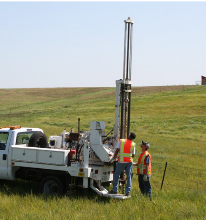
KDOT employees Rick Hinderliter and Derek Surber conduct a geology survey along U.S. 281 in Russell County to gather information for the upcoming modernization project.
